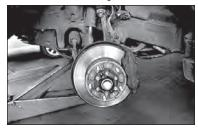
Lug nuts must be tightened in a star or crisscross pattern to ensure uniform pressure and alignment. Apply torque evenly by repeating the star or crisscross pattern until desired torque is reached.
